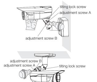
3. Tighten the tilting lock screw.
