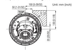
\* The above figure indicates the available area to fix the wire lug plate when installing the camera. Determine the position to fix the wire lug plate in this area.
