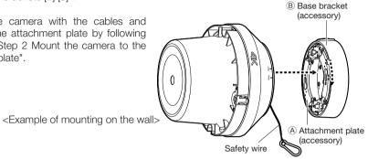
(5) Hitch the hook at the tip of the safety wire to the wire lug plate fixed on a ceiling or a wall.
