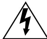
The lightning flash with arrowhead symbol, within an equilateral triangle, is intended to alert the user to the presence of uninsulated "dangerous voltage" within the product's enclosure that may be of sufficient magnitude to constitute a risk of electric shock to persons.
