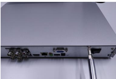
1. Loosen the screws of the upper cover and side panel.
