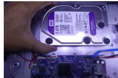
3. Place the HDD in accordance with the four holes at the bottom.
